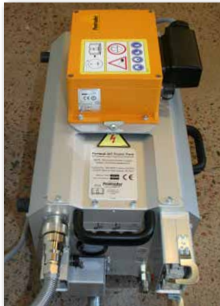
Easy fitting of Wireless Remote Control and Receiver on Pentpak if no Transport Trolley is used
