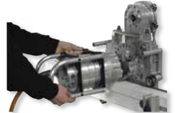
Easy removal of HF-motor
