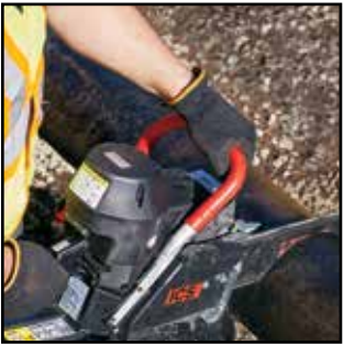
Cut up to a 10" (25cm) pipe from one side.
