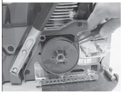
7.3 Remove clutch shield with small screwdriver.
