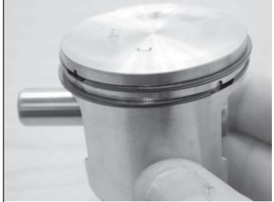
13.15 Align piston in correct orientation.
