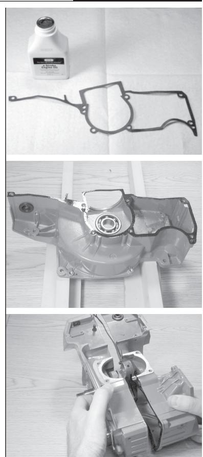
20.18 Align crankcase gasket on flywheel side crankcase pins.
