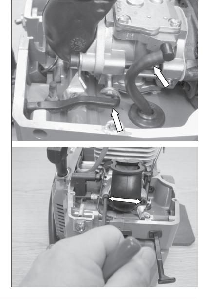
12.3 Remove carburetor attachment screws.
