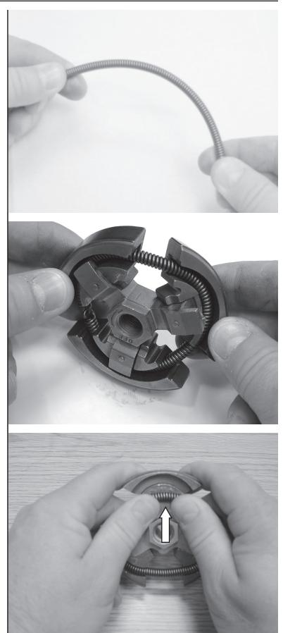
7.8 Assemble clutch shoes as shown.
