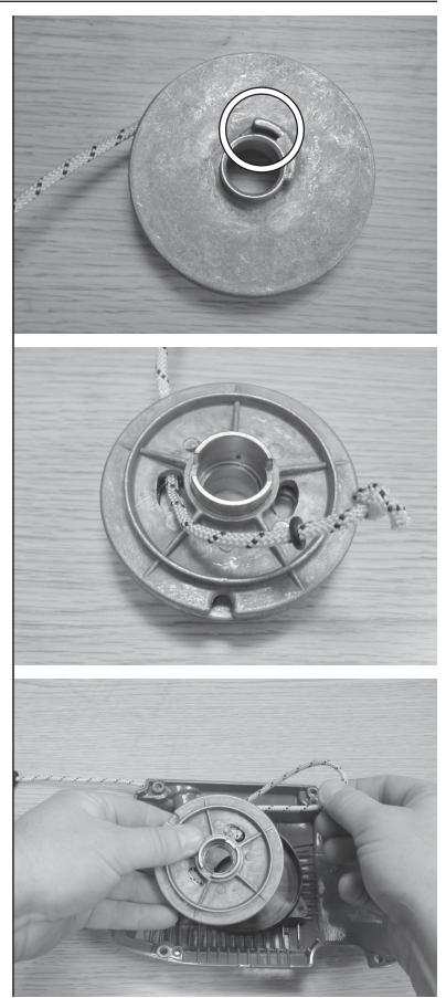
8.11 Install starter rope and tie knot.
