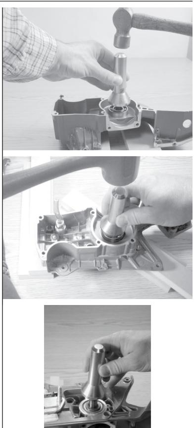
20.15 Install crankshaft into clutch side of case.
