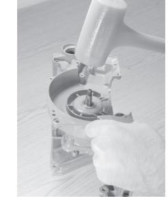
20.5 Remove the flywheel side of crankcase seal.
