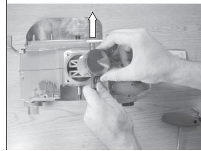
13.4 Remove wrist pin retaining clips
